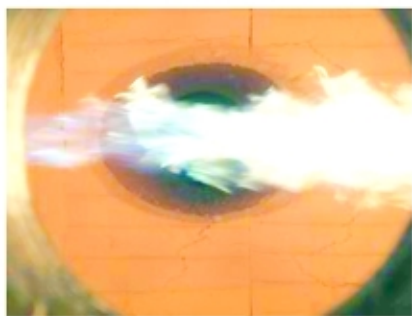
Flameless oxyfuel burner Rebox-W, mounted to the left in the photographs, firing in flame mode (<800° C) in the photograph to the left and in flameless mode (>800° C) in the photograph to the right.
