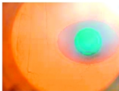
Flameless oxyfuel burner Rebox-W, mounted to the left in the photographs, firing in flame mode (<800° C) in the photograph to the left and in flameless mode (>800° C) in the photograph to the right.
