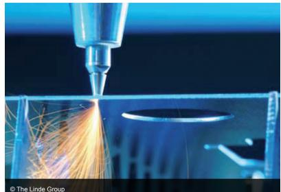
Laser cutting uses light as heat and is the most accurate of all the processes.
